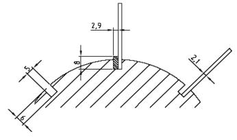
After several reblading operations on the same cylinder it is recommended to increase the copper width slightly. Mostly it is sufficient to increase width by one decimillimeter (0,1 mm). In our example the copper measurements would become 3,0 mm wide x 8,0 mm high. In order to facilitate easier entry of the caulking material into the grooves, wedge-shaped copper strip at its upper edge has to be increased by 0,2 mm, whereas the width at the bottom edge has to be reduced by 0,2 mm.
